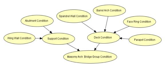
Figure 3. A representative BBN model for masonry arch bridges
