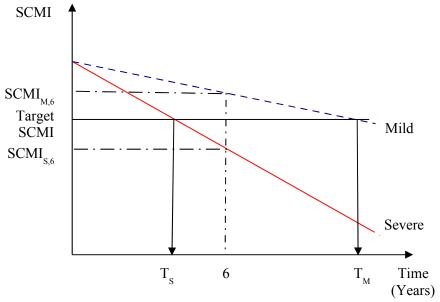
Figure 2. Inspection interval for mild and severe environment group bridges
