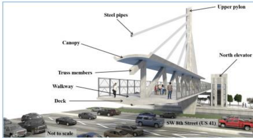
Figure 6. Cross-section rendering of pedestrian bridge, north view. (Source: FIU, modified by NTSB)
