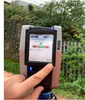
Setting the Laser Scanner on Site (Inclinometer, Quality, Resolution)
