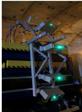
Figure 6. Mechanical installation of an inspection arm holding six sensors.
