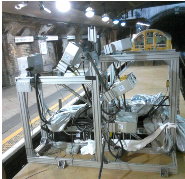
Figure 2. Metal frame with six sensors on flat wagon. Assembly photograph
