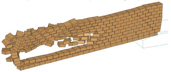
(c) Low unit-mortar adhesion at 600mS (V80-H1800-T400-W@600mS)
