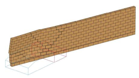
(a) Thin wall with high unit-mortar adhesion at 85mS (V80-H1800-T200-S@85mS)
