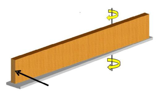
Figure F1 Assumed mode of response of parapet
