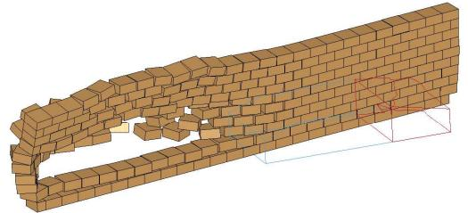
(b) Low unit-mortar adhesion at 405mS (V80-H1800-T400-W@405mS)
