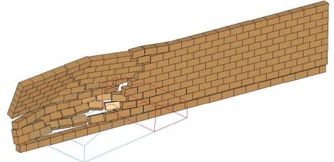
(b) Thin wall with high unit-mortar adhesion at 145mS (V80-H1800-T200-S@145mS)
