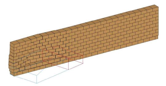
(a) Low unit-mortar adhesion at 105mS (V80-H1800-T400-W@105mS)
