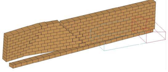
(c) Medium unit-mortar adhesion at 430mS (V80-H1800-T400-M@430mS)
