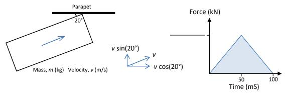
Figure B1 – Calculation of applied impulse
