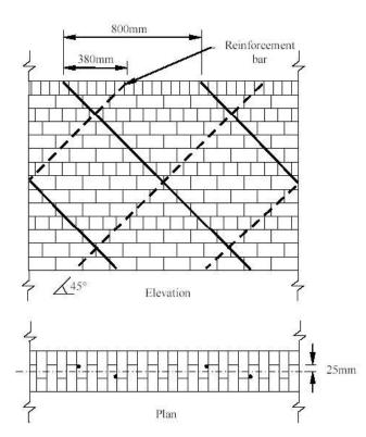
Figure 4 Example diagonal bar reinforcement layout
