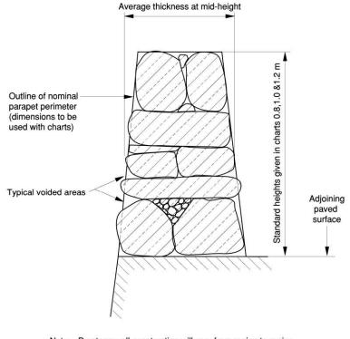
Note: Drystone wall construction will vary from region to region and this diagram should be considered diagrammatic only.
