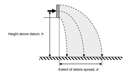
Figure 5 Extent of debris spread: definition
