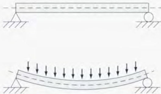
Figure B.42 – A simply supported beam bending under a distributed lateral load
