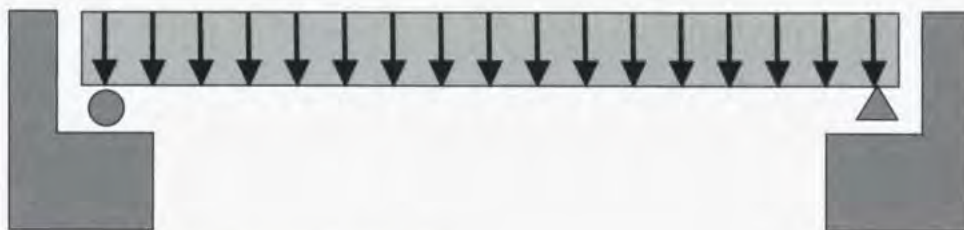
Figure B.35 – Dead load on a bridge [9]
