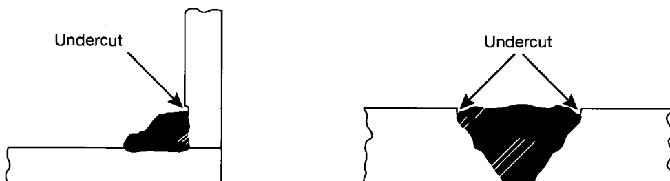
Figure D.5 – Undercut weld [36]
