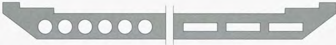
Figure B.7 – Typical cross-sections of voided slab bridges
