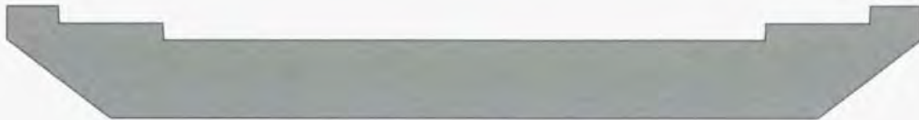
Figure B.6 – Typical cross-section of a solid slab bridge
