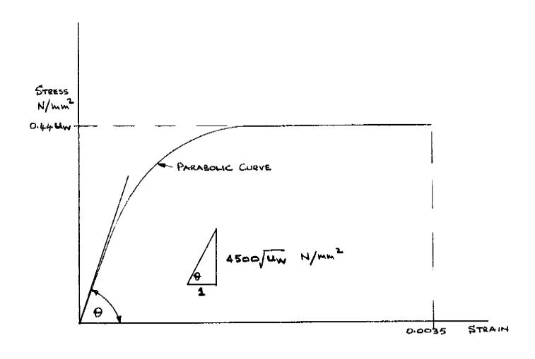
FIGURE 2. SHORT TERM DESIGN STRESS-STRAIN
